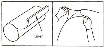
"PS" adhesive is pressure sensitive and sticks to anything with which it comes in contact. During application, the release liner must be removed. Protect the film and exposed adhesive during the entire installation procedure. Do not let it touch anything but the glass on which it is to be installed.
